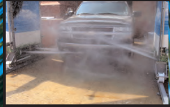
Rocker Panel Blaster includes nose and tail creep feature ensures that adequate time is spent on commonly "hard-to-clean" areas
